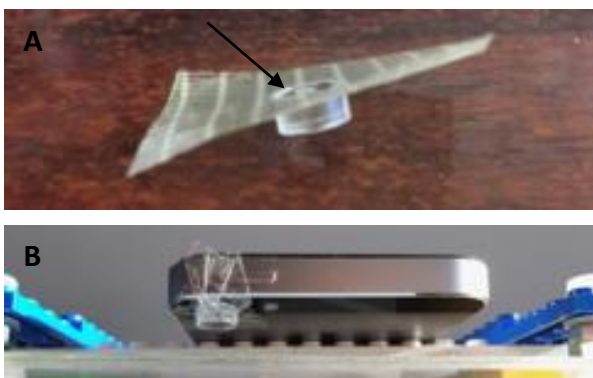
Figure 2 (A) Tape attached to the rim of the lens. The hole cut just fits over the lens rim. (B) Lens positioned on the phone and held in place with tape.
