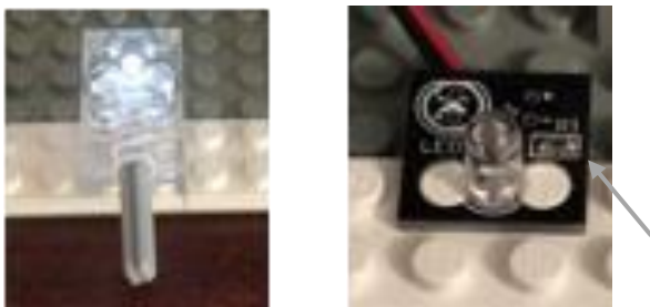
Figure 5. Left: a clear Lego™ brick with LED and battery fitted inside the brick. Right: PCB with LED and minuscule resistor (arrowed) fitted onto the studs of a Lego™ plate.
